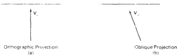
Figure 12-17 Orientation of the projection vector V_p to produce an orthographic projection (a) and an oblique projection (b).
