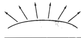
Figure 14-4 Diffuse reflections from a surface.
